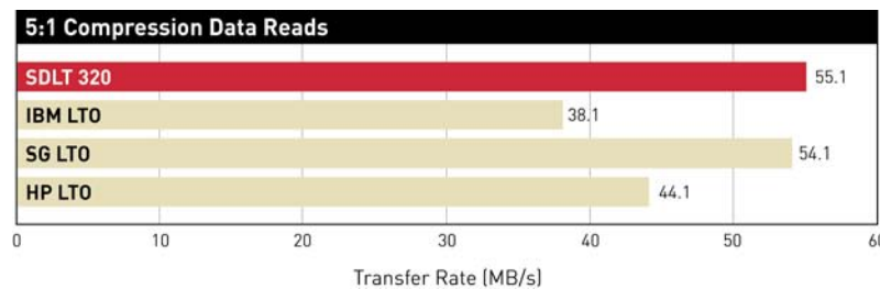
Figure 3 - In read data transfer tests the SDLT 320 read data 44% faster than the IBM 3580 Ultrium and 24% faster than the HP Ultrium 230.
